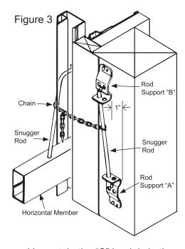
4. After makin certain the "S" hook is in the proper link (latched chain should be about 6" from top of horizontal member) close the "S" hook slightly so it will not become detached from chain.
