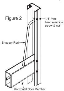
Before installing the second half of the snugger to the face of the door jamb, close the door (door must have a center stop, or otherwise be held stationary).
